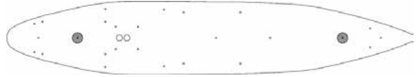
Weight Bolt Installation (Legend Area Highlighted)
